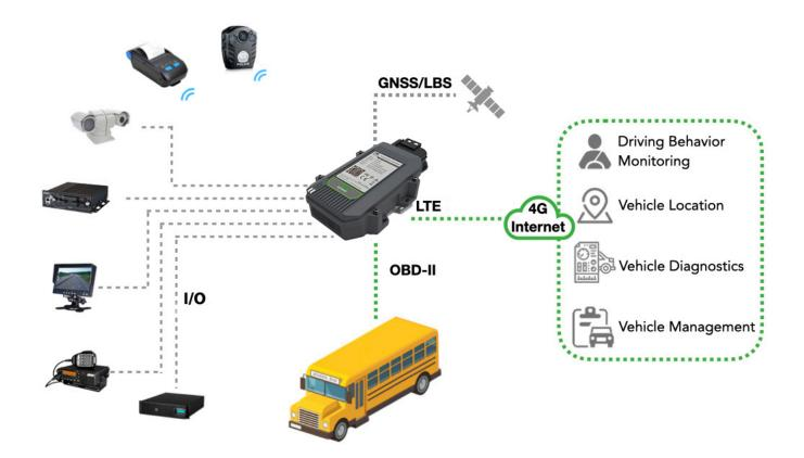
Featuring extensive I/O, standard protocols for communications and vehicle diagnostics, the VT310 can be connected to multiple peripherals on board, constantly collects data from different parts of the vehicle, secures uninterrupted communications between vehicles and the management center, reports problems once detected, ensuring safe and efficient running of vehicles and business.
